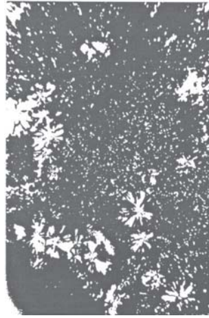
Fig. 6c. PP M_w = 320\ 000 with Irgastab NA 04
