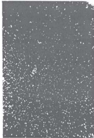
Fig.6b. PP M_w = 320\ 000 with Irgastab NA 21
