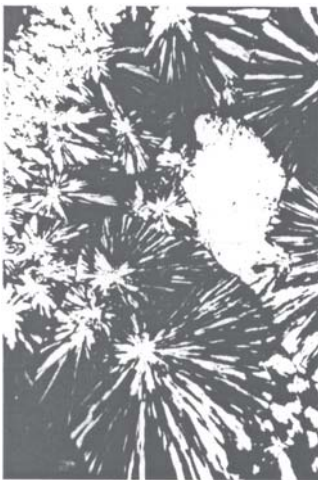
Fig.7a. PP MFI = 2.5 g/10 min., without nucleating agent
